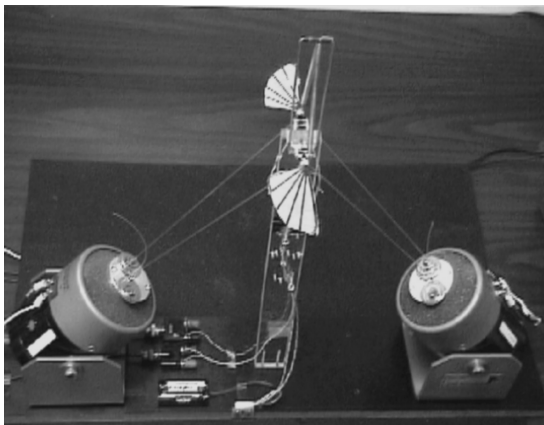
Fig. 9 Shaker-actuated testbed designed to provide control of vibratory wingbeat patterns.
